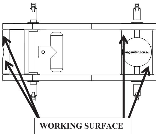
\* Max Breakaway determined in laboratory environment on 2" thick SAE1018 Steel with surface roughness 63 micro inches. Many factors contribute to the actual breakaway force in each application. Always test the magswitch in each application before deployment. Refer to the magswitch information booklet for more information.
