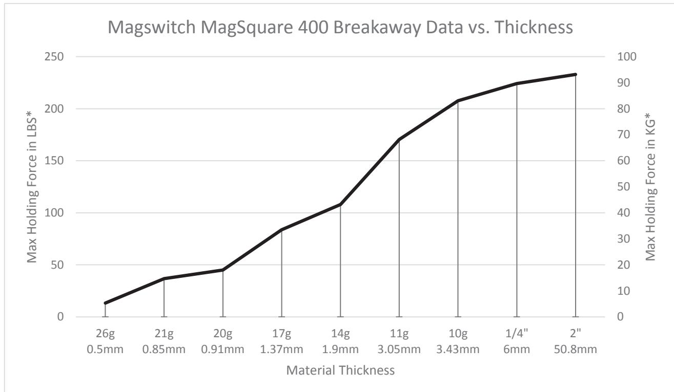
\* Max Breakaway determined in laboratory environment on 2" thick SAE1018 Steel with surface roughness 63 micro inches. Many factors contribute to the actual breakaway force in each application. Always test the magswitch in each application before deployment. Refer to the magswitch information booklet for more information.
