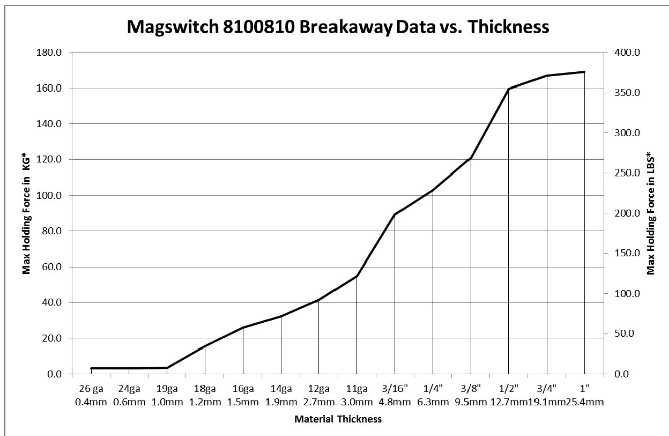
\* Max Breakaway determined in laboratory environment on 2" thick SAE1018 Steel with surface roughness 63 micro inches. Many factors contribute to the actual breakaway force in each application. Always test the magswitch in each application before deployment. Refer to the magswitch information booklet for more information.
